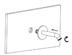
3. Push back plate to the wall surface. Ensure o-ring is firmly gripping the spout and creating a tight seal. Use silicone to seal the back plate.
