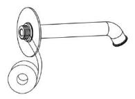
2.Twist the spout clockwise on and hand tighten.
